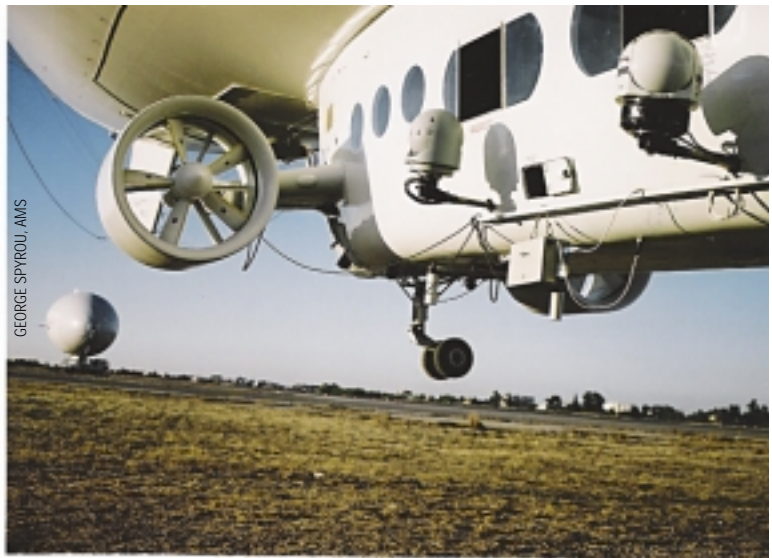
These two AMS airships are equipped with MX-15 cameras, which were used in the 2004 Summer Olympic Games security operations.
